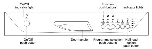
**Function push buttons:** in addition to the dishwashing programme selected, the following functions can also be set with the help of these buttons: water softener setting, deactivation/activation of the inflow of rinse aid and the cancelling of a programme in progress.
